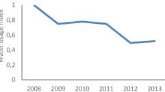
In the case of pre-treating the metal strip prior to coating, two alternative technologies are available. The traditional method of pre-treatment of using a spray bath to deposit the conversion coating on the surface of the metal strip has been largely superseded by the so-called "no-rinse" technique, in which the chemical agent is applied by roller-coating, requiring significantly less water
