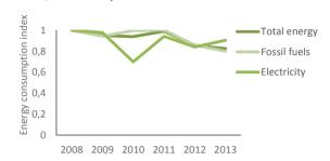
The focus on energy efficiency has been successful. For example, installation of more efficient VOC destruction systems (Regenerative Thermal Oxidisers), upgrading the curing oven configuration and optimising the overall process management on the coil coating lines have helped decrease the total energy consumption by 17% since 2008.
